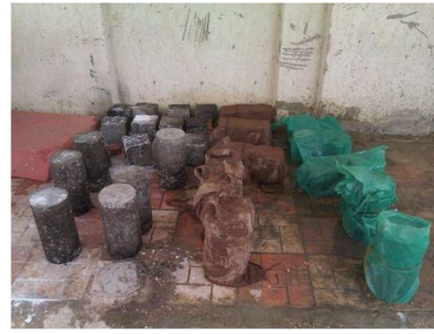
b) Curing the specimens with the five methods
