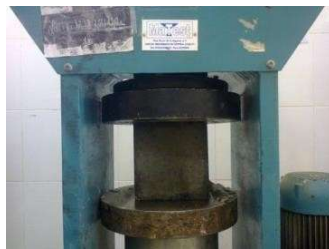
a) Test setup for compressive strength
