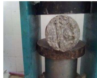
b) Test setup for Indirect tensile strength
